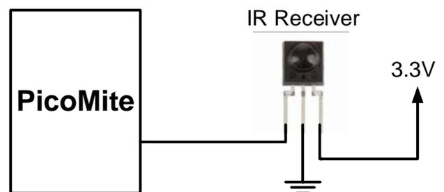
IR remote controls can address many different devices (VCR, TV, etc) so the program would normally examine the device code first to determine if the signal was intended for the program and, if it was, then take action based on the key pressed. There are many different devices and key codes so the best method of determining what codes your remote generates is to use the above program to discover the codes.
