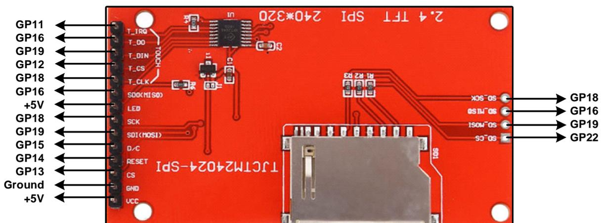
To match the above connections the following configuration commands should be entered, one by one at the command prompt:
