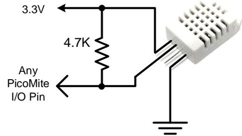
To get the temperature or humidity you use the HUMID command with three arguments as follows:
