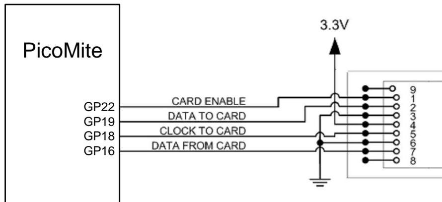
Note that you can use many different configurations using various pin allocations – this is just an example based on the configuration commands listed above.
