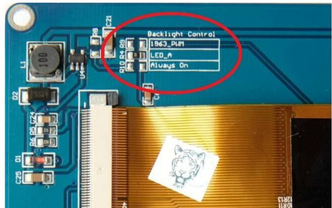
However, it is better to use the SSD1963 controller to generate this signal as it frees up one I/O pin. To use the SSD1963 for brightness control the zero ohm resistor should be removed from the pair marked "LED-A" and used to short the nearby pair of solder pads marked "1963-PWM". The PicoMite can then control the brightness via the SSD1963 controller using the BACKLIGHT command.
